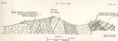
FIG. 40. Section across South-west Part of Ardnamurchan Igneous Complex 1, Highland Schists; 2, Trias; 3, Lias; 4, Inferior Oolite (limestone and sandstone); 5, Tertiary basalt lavas; 6, Outer cone-sheets of Centre 2; 7, Inner cone-sheets of Centre 2. Ring-dykes a, c, e, f, g and A as lettered on Fig. 38, p. 81.
